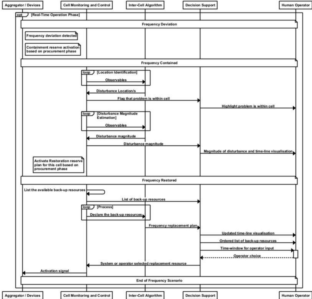
Fig. 3. Scenario 1) Single frequency event sequence diagram.
