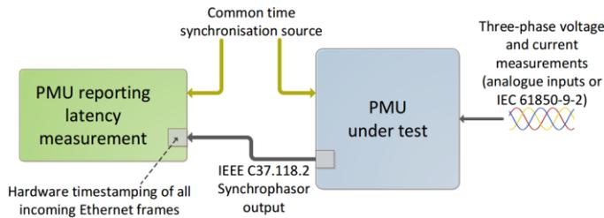
**Figure 7: Overview of PMU reporting latency measurement method**
