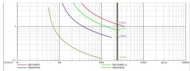
**Figure 11: Relay operating times (adaptive settings)**
