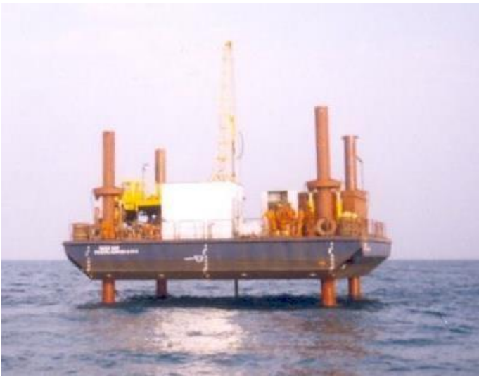
FIGURE 1: JACK-UP WITH CYLINDRICAL LEGS (MS CYBERMARINE TECHNOLOGIES PTE. LTD.)
