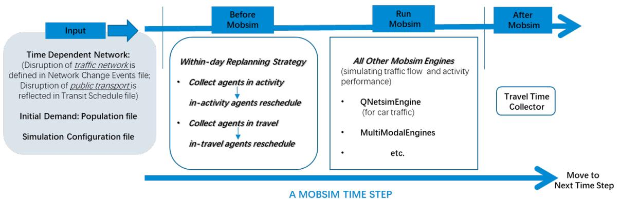
Fig. 1. Building block of Within-Day Replanning Module.
