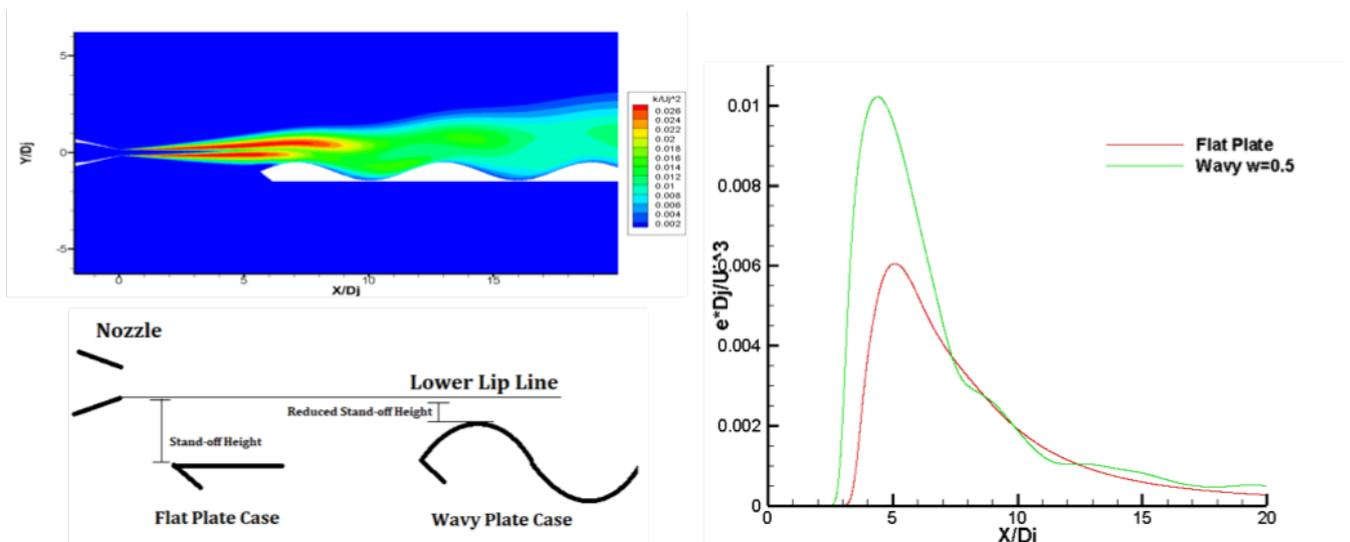
Figure 1: Normalized TKE using STAR-CCM+ as solver and  $k - \epsilon$  realizable turbulence model)
