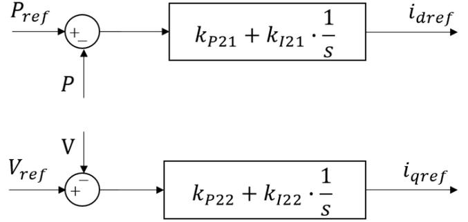
Figure 3 Power and voltage control
