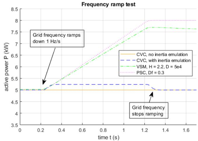
Figure 14 Frequency ramp test
