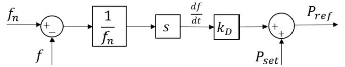
Figure 4 Inertia emulation loop
