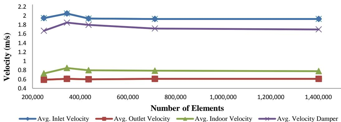
Figure 9 Comparison of solutions from various grid adaptation methods. The variables are the average velocity at the inlet and outlet of the wind towers and interior of the test room
