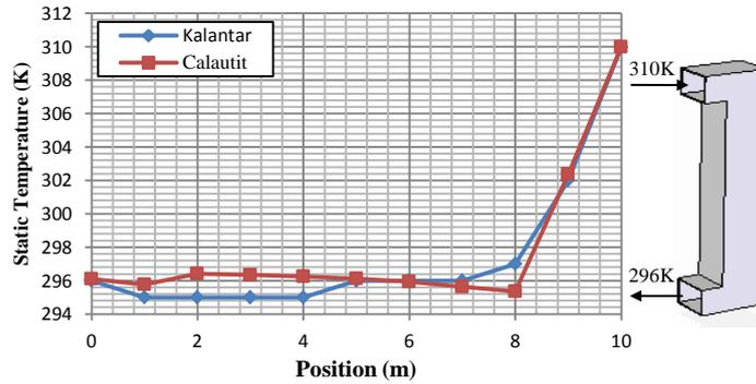
Figure 13 Comparison of the airflow temperature variation from inlet to outlet obtained from the CFD results from the two studies.
