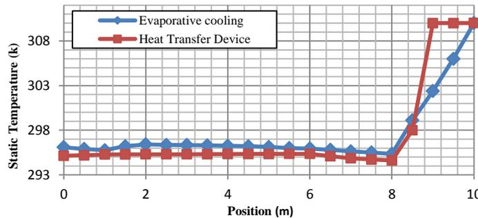
Figure 14 Comparison of the variation of temperature of airflow from entering to exiting.
