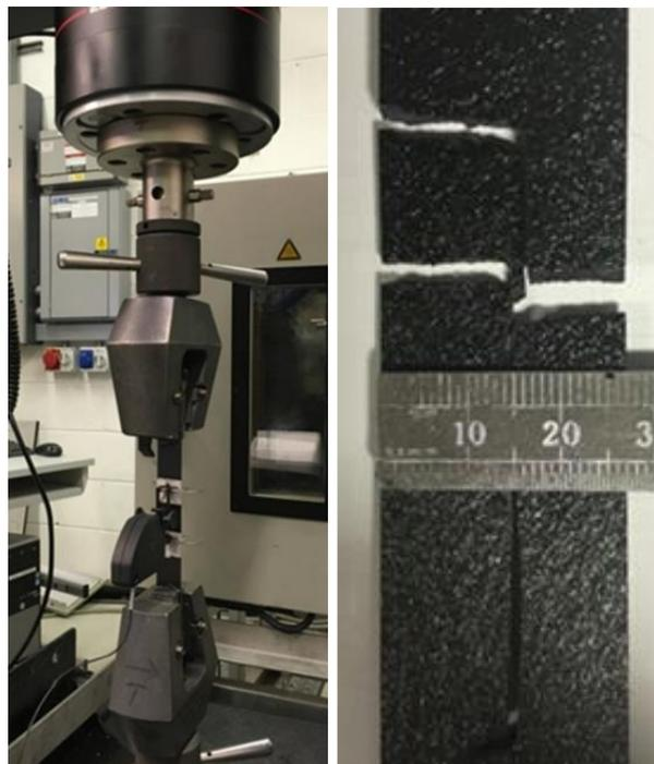
Figure 3 Tensile testing setup and typical fracture cross section of 3mm fibre laminate composite specimen
