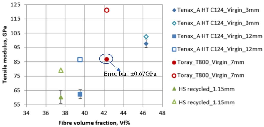
Figure 9 Experimental (solid marker) and predicted (hollow marker) tensile properties of composites reinforced with 3mm,7mm and 12mm aligned fibre tapes and 1.15mm aligned recycled fibre tapes
