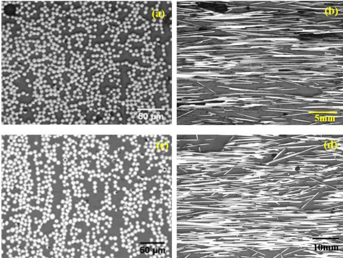
Figure 6 Micrograph of aligned composite cross section and in-plane view:
