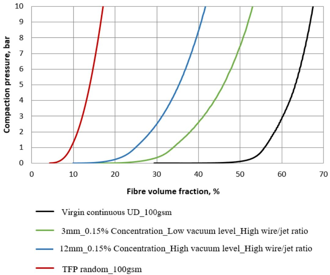
Figure 5 Dry fibre tape compaction test results
