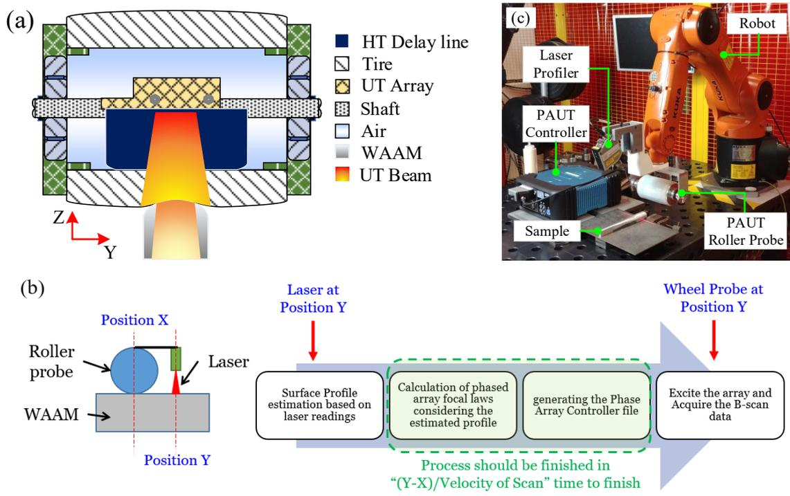
Figure 1 (a) A simplified design of the WAAM high temperature PAUT roller probe, (b) integrated robotic system for the inspection of WAAM including the roller probe, PAUT controller and the laser profiler, and (c) plan for laser-assisted on-line correction of PAUT focal laws as the roller probe scans a sample with changing surface profile
