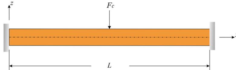
Fig. 3. Clamped beam subjected to a central point force.
