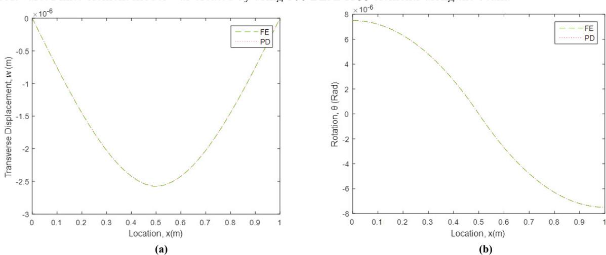
Fig. 2. Variation of (a) transverse displacement, (b) rotation along the beam (PD: Peridynamics, FE: Finite Element Analysis).
