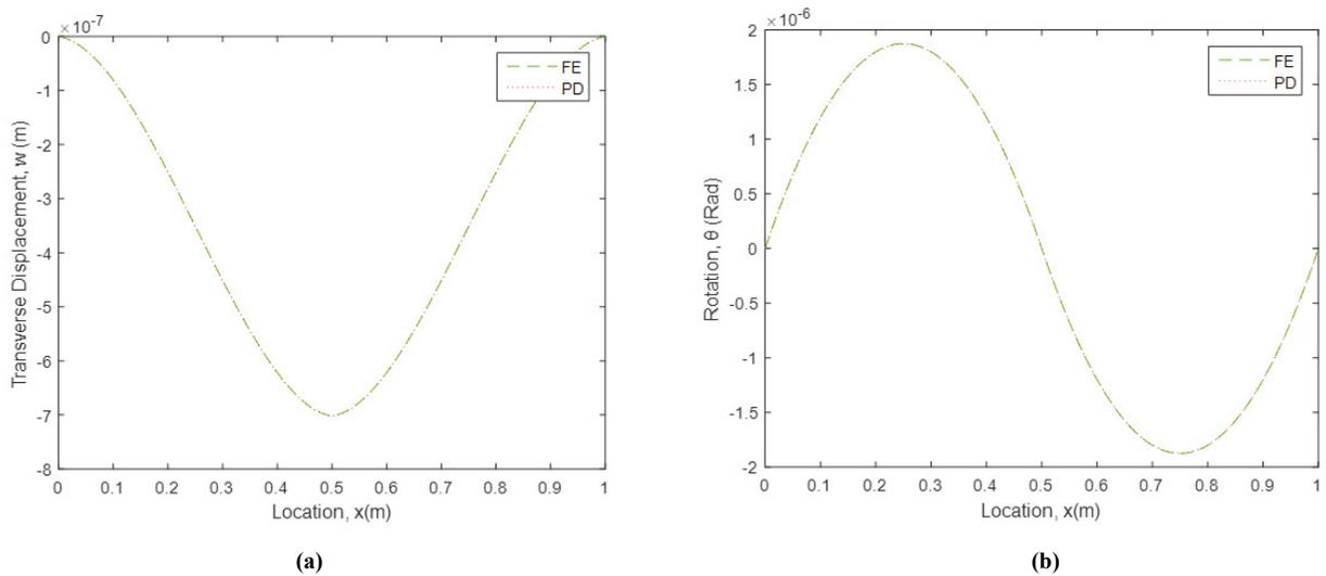
Fig. 4. Variation of (a) transverse displacement, (b) rotation along the beam (PD: Peridynamics, FE: Finite Element Analysis).
