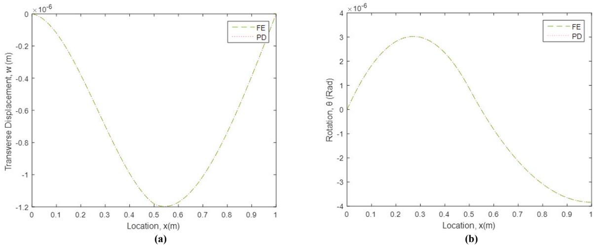
Fig. 6. Variation of (a) transverse displacement, (b) rotation along the beam (PD: Peridynamics, FE: Finite Element Analysis).
