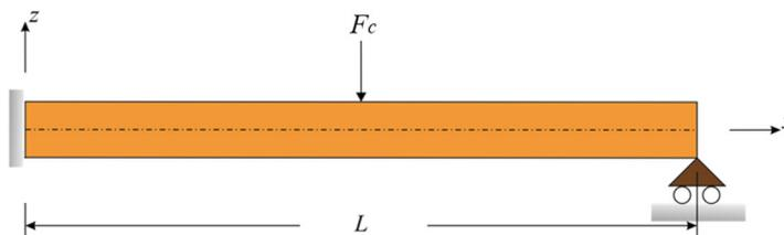
Fig. 5. Beam subjected to a central point force and mixed boundary conditions.
