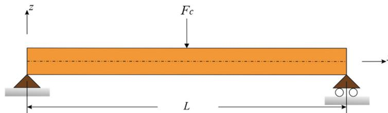
Fig. 1. Simply supported beam subjected to a central point force.
