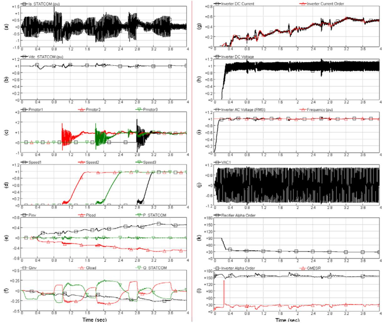
Fig. 3 Simulation results of black start and various load switching, (a): STATCOM AC current; (b) STATCOM DC link voltage; (c) Induction machine active power; (d) Induction machine speed; (e) Active powers of HVDC inverter, load and STATCOM; (f) Reactive powers of HVDC inverter, load and STATCOM; (g) HVDC converter DC currents; (h) HVDC inverter DC voltage; (i) Network AC rms voltage and frequency; (j) Network AC voltage; (k) Rectifier alpha order; (l) Inverter alpha order and gamma measurement
