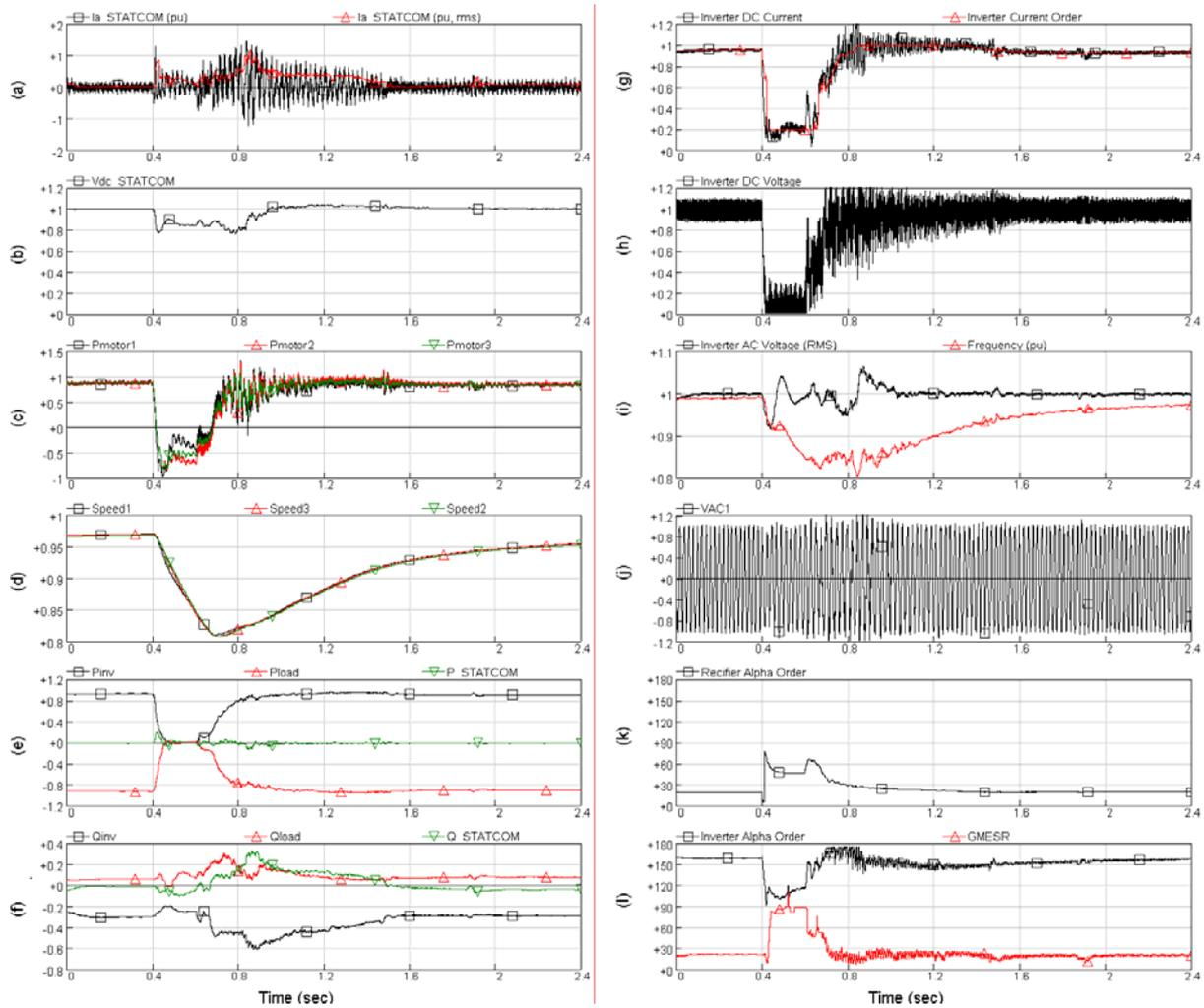
Fig. 4 Three-phase to ground fault on rectifier side (same axes as in Figure 3)
