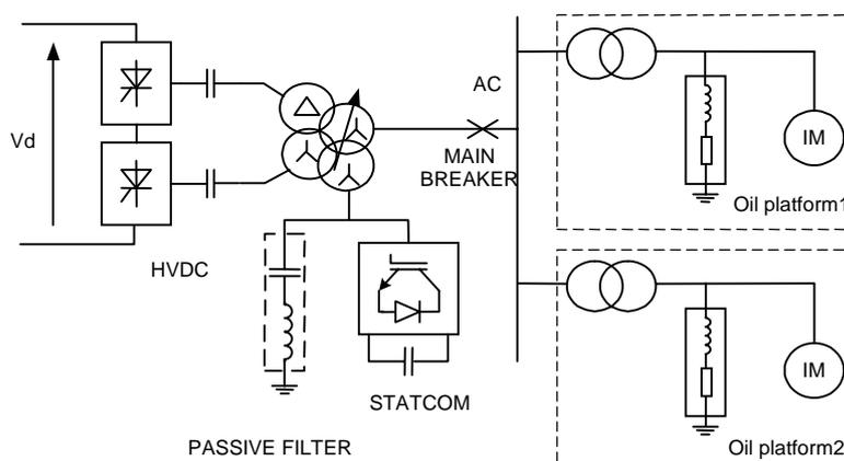
Figure 1 Schematic diagram of hybrid HVDC system supplying power to offshore oil platforms
