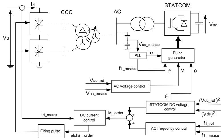
Fig. 2 Schematic diagram of the control strategy
