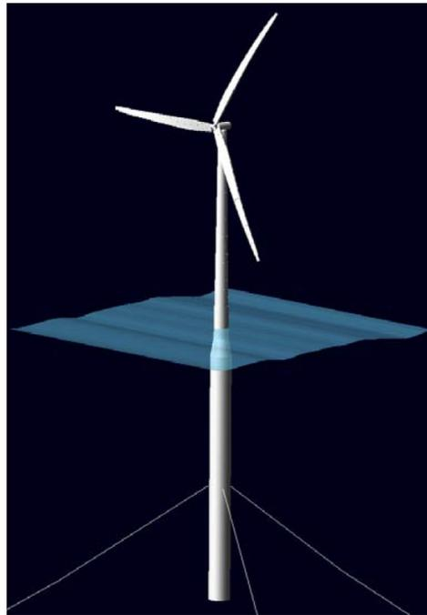
Figure 6. The OC3 floating spar-buoy wind turbine system [63].
