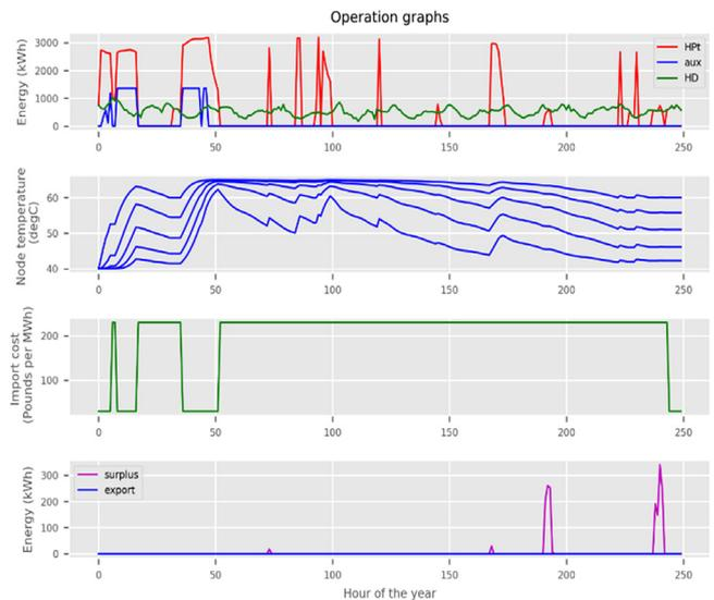
Fig. 2. Operational graphs output for MPC and wind tariff over a windless winter 10-day period.
