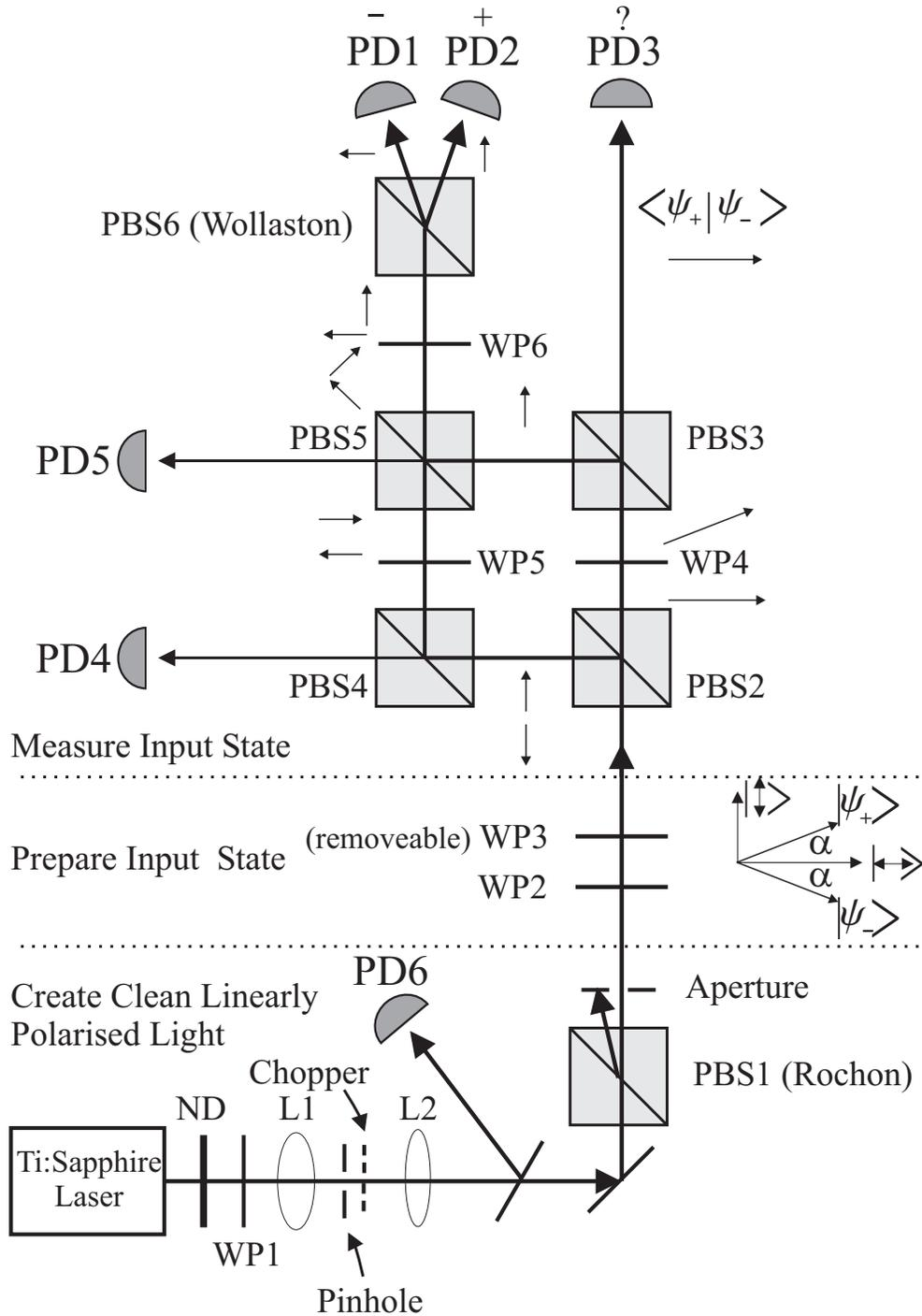
FIG. 2. Experimental setup to prepare, process and discriminate the states  $|\psi_+\rangle$  and  $|\psi_-\rangle$ . See text for full description. L = lens, ND = neutral density filter to attenuate the light, PD = photodiode, WP = waveplate, all  $\lambda/2$ , to rotate the polarisation of the light. PBS = polarising beam splitter, all reflect vertical polarisation and transmit horizontal polarisation.
