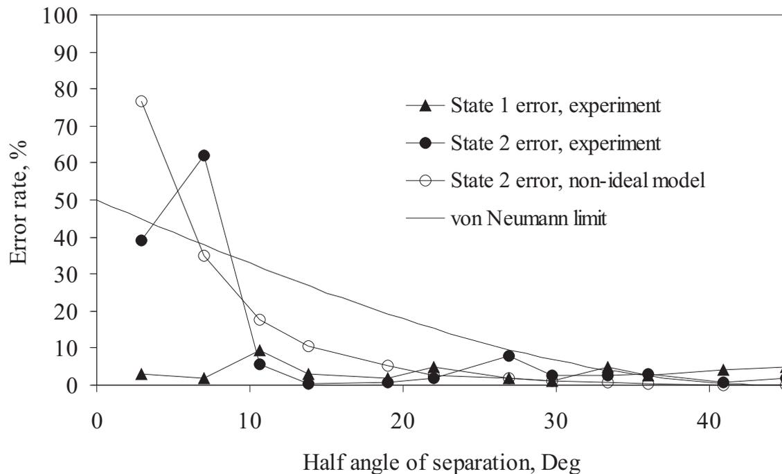
FIG. 4. The experimentally observed error rates (PD2 and PD1) obtained with input states  $|\psi_+\rangle$  and  $|\psi_-\rangle$  respectively. Also shown is the theoretical model using non-ideal beamsplitters with the same characteristics as in the experiment, and the best possible von Neumann error rate.
