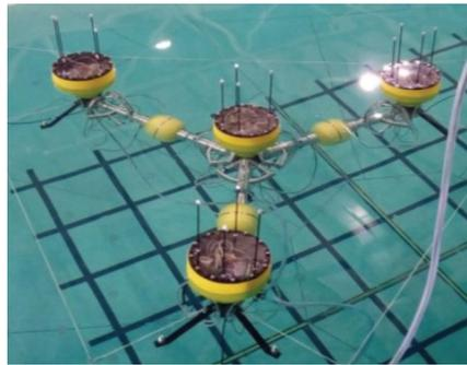
Figure 1 layout of a WEC array
