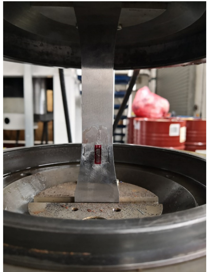
Fig. 3. Uniaxial fatigue specimen undergoing fatigue testing.
