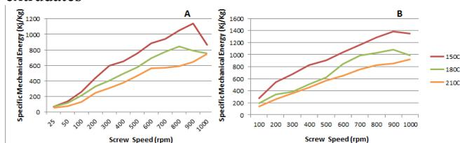
Figure 3: Specific mechanical energy curve for A) Affinisol™ and B) Plasdone™ S630
