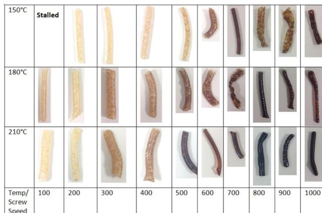
Figure 1: Physical appearance of Affinisol™ HPMC HME 15LV polymer extrudates
