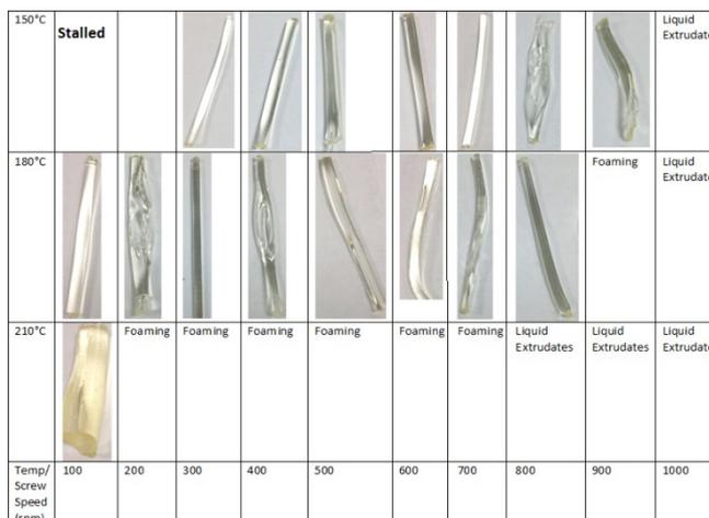
Figure 2: Physical appearance of Plasdone™ S630 polymer extrudates
