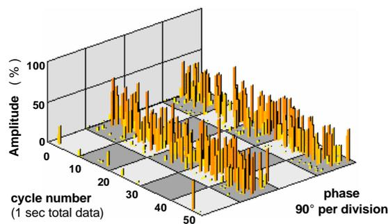
Figure 12: UHF PD Signals from Sensor S1, Phase-Resolved to the 50 Hz Power Frequency
