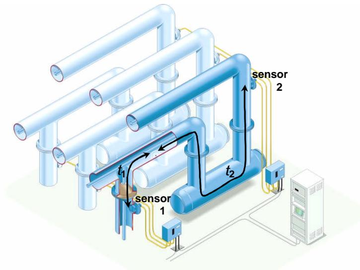
Figure 2: Locating a PD Source in a GIS by the Time-of-Flight Method
