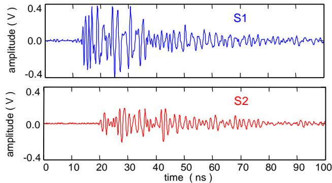
Figure 7: Time-Domain UHF Signals Recorded Simultaneously at Two Sensors
