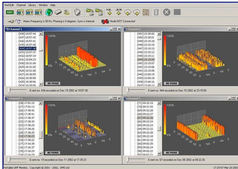
Figure 15: Examples of PD Patterns Recorded at Different Stages During the Monitoring Period
