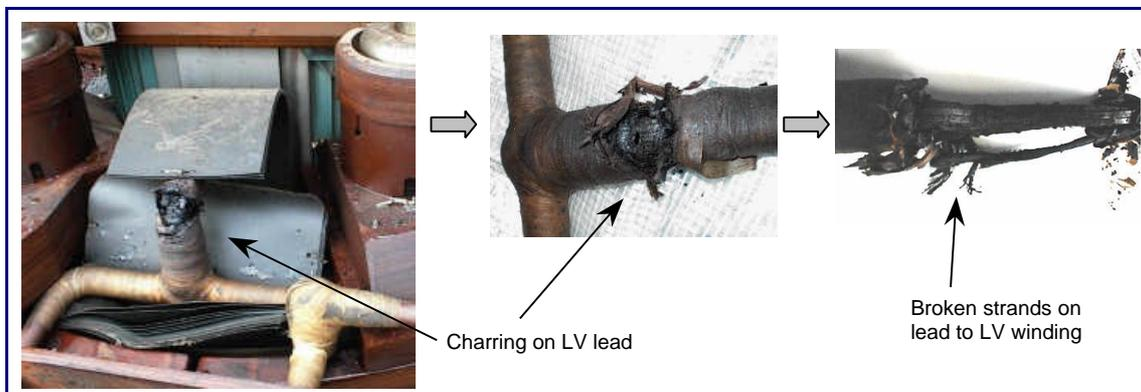
Figure 16: Damaged Joint on 33 kV Lead
