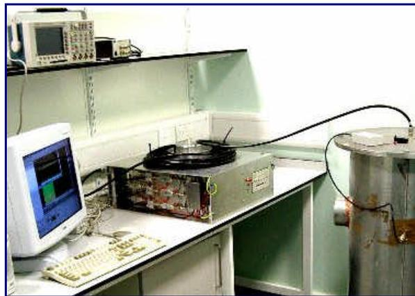
Figure 17: Portable UHF Transformer Monitoring Unit in Development
