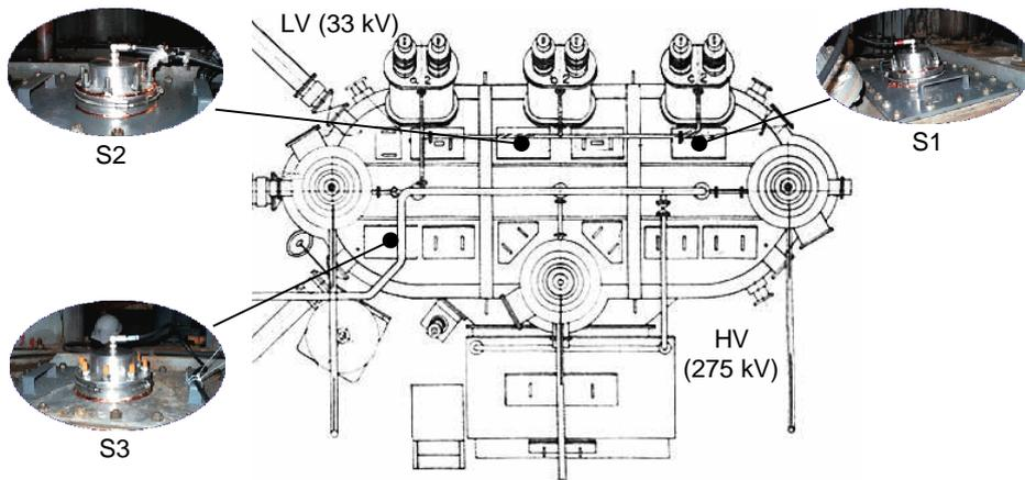
Figure 14: Top View of the 120 MVA 3-Phase Transformer Equipped for UHF Monitoring
