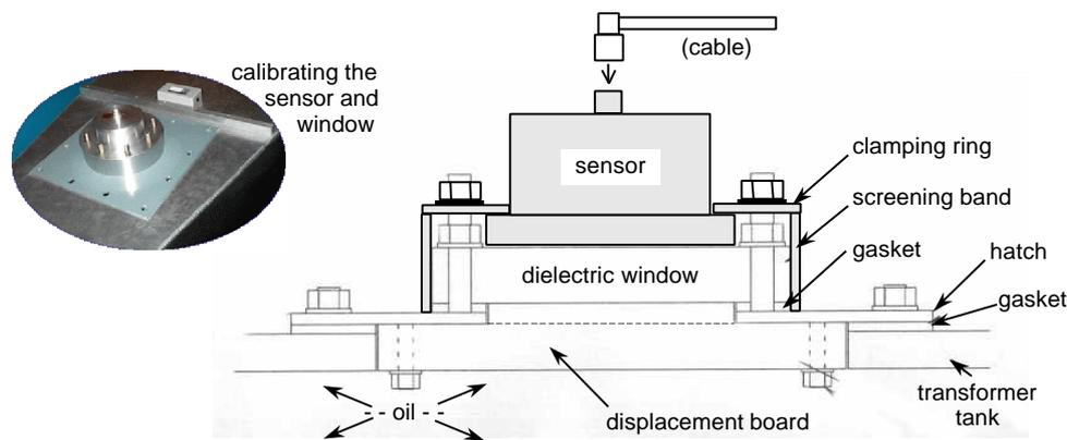
Figure 4: UHF Sensor Assembly on a Transformer Hatch Cover
