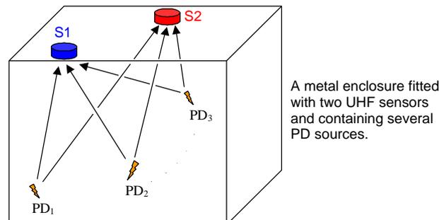
Figure 6: Recognizing Multiple Signal Sources Using Two or More UHF Sensors
