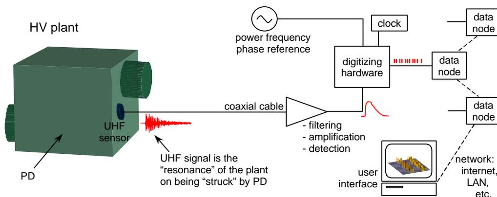
Figure 1: Basic Principles of UHF Condition Monitoring
