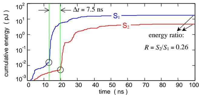
Figure 8: Cumulative Energy Plots Illustrating Parameter Extraction for a UHF Signal Pair
