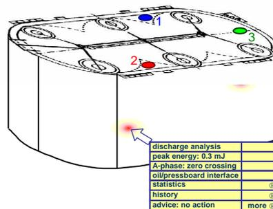
Figure 3: Graphical Interface for Accessing Transformer Monitoring Information
