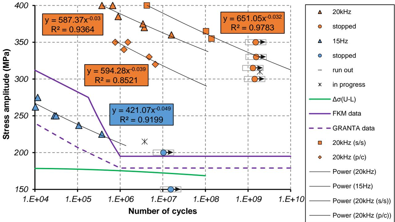
Fig. 4 Summary of fatigue testing for S275JR+AS including base dry and pre-corroded samples.
