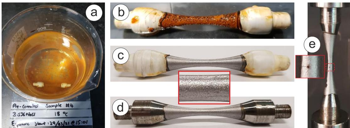
Fig. 3 Pre-corroded specimen for ultrasonic test: a) 3.5% NaCl solution with the submerged specimen; b) rust layer on the specimen; c) washed specimen with thread seal tape; d) specimen ready for testing; e) specimen at the end of the test with a crack in the middle.
