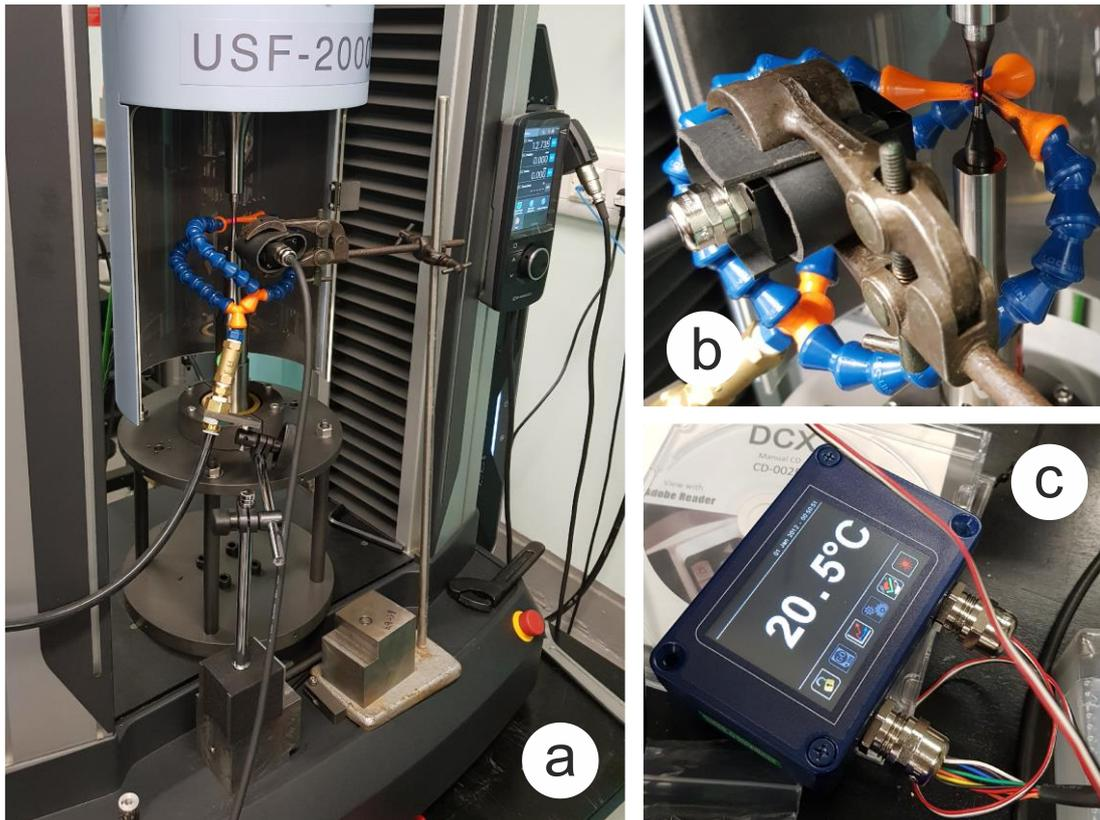
Fig. 1 Arrangement for temperature control of the ultrasonic test: a) USF-2000A with average stress loading mechanism; b) Pyrocube IR temperature sensor; c) touch screen display for PyroCube.
