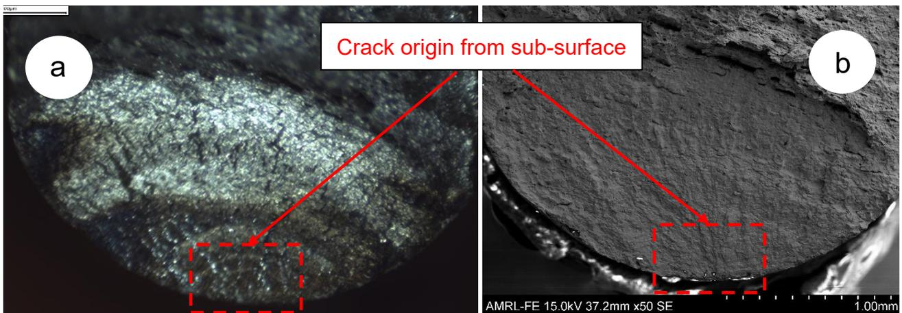
Fig. 6 Investigation of the fracture surface of the sample run at 400 MPa stress amplitude with a sub-surface crack origin for over 4 million cycles using: a) optical microscopy; b) SEM microscopy.
