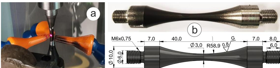
Fig. 2 Specimen for ultrasonic test: a) inserted in UFS-2000A with temperature measurement spot; b) solid model with dimensions and manufactured and painted.
