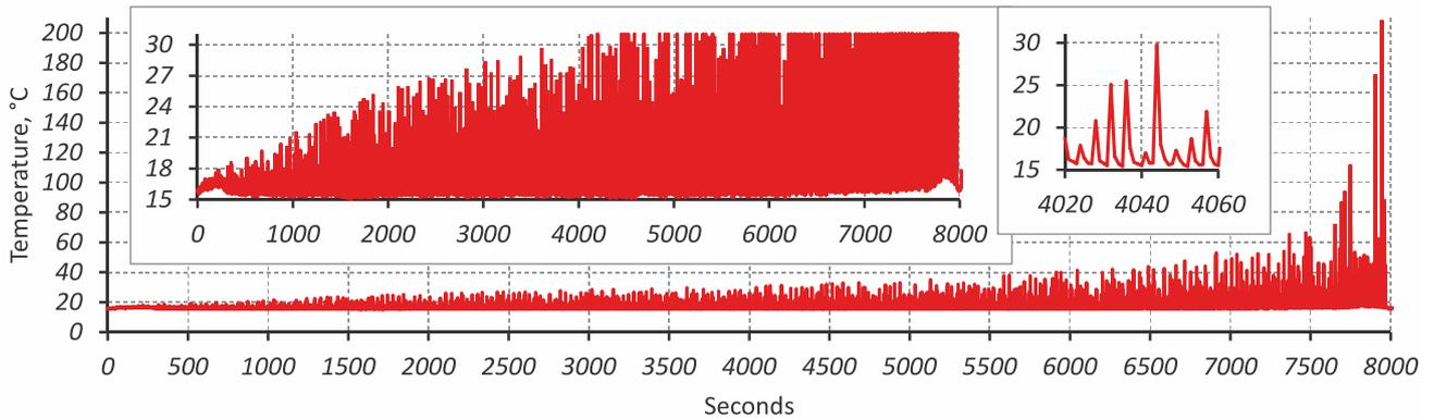
Fig. 5 Temperature history of the ultrasonic fatigue test lasted 4m cycles at 400 MPa stress amplitude.
