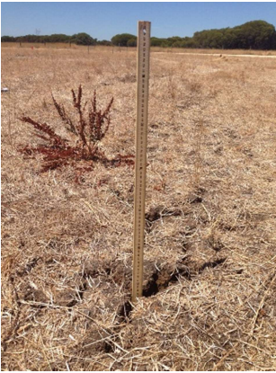
Figure 4 Flat lying land, showing extreme desiccation cracks posing a challenge in the baked hard clay soil for various surface monitoring techniques.
