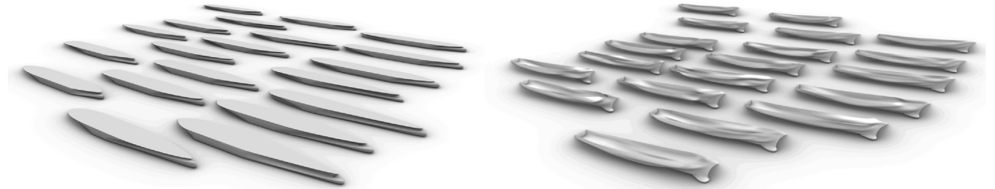
Fig. 3. Three dimensional design variations of the PD hull (on the left) and DTMB 5415 hull (on the right) generated with 26 and 27 design parameters defined using PD- and GMF-based parameterisation, respectively. These design variations can also be visualised in a video at https://bit.ly/3BiB9wZ . For PD hull, parameterisation is performed on the submerged part below the waterline, and for both hull their geometric moments are evaluated for the submerged part.
