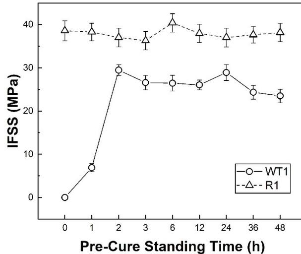
Figure 6: Apparent IFSS versus pre-cure standing time
