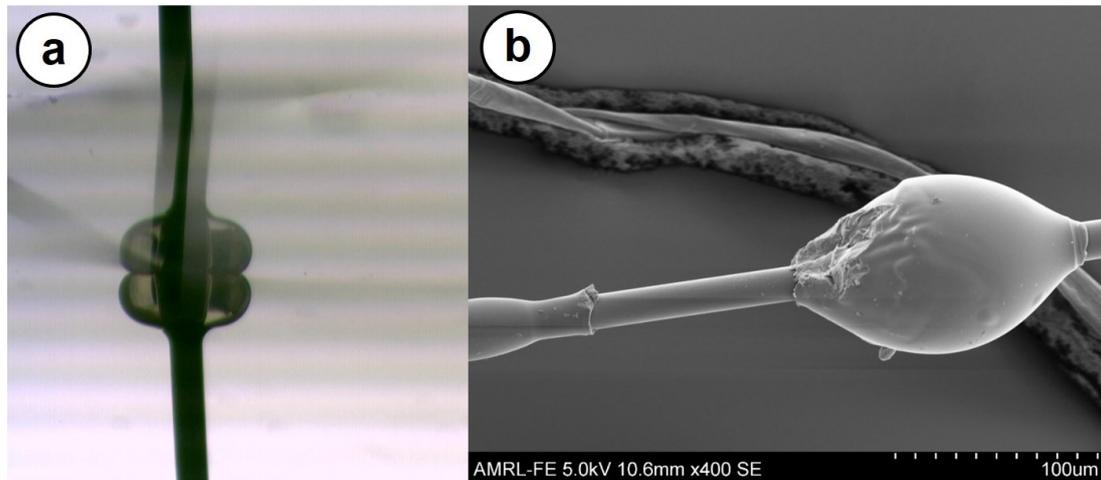
Figure 2: (a) In-situ micrograph of WT1 droplet (b) Post-test SEM of R1 droplet
