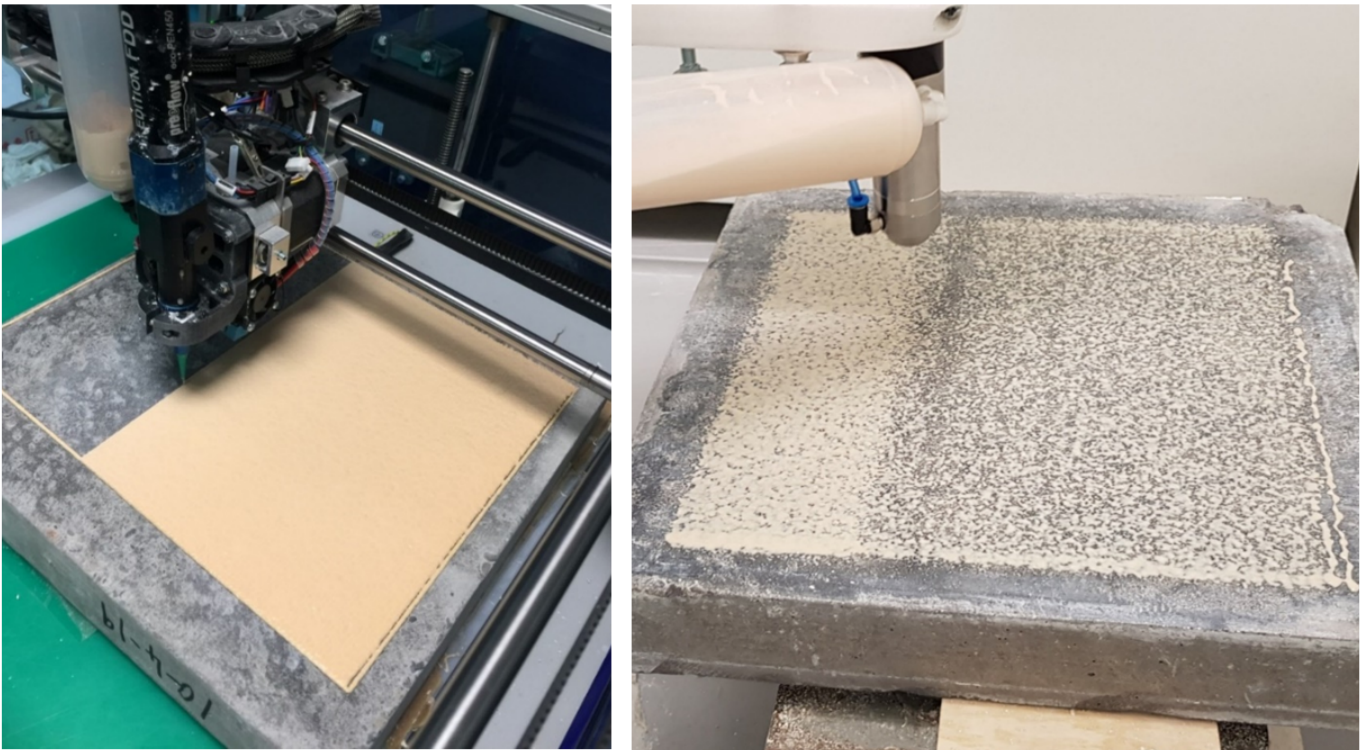
Fig. 4. The (left) 3D printing and (right) robotic spray coating of AAM onto concrete slabs.
