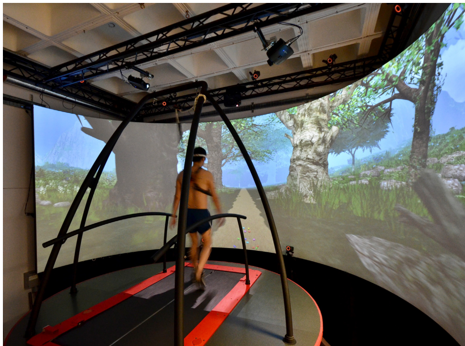
Figure 2 The Motek CAREN system with a treadmill system, safety harness for patient and a large virtual reality screen. The system is equipped for 3D Gait analysis, whilst the patient navigates a virtual environment. This can test a patient's gait whilst they perform activities of daily living.
