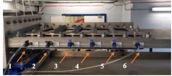
Figure 4: Pressure taps distribution numbered from 1 to 6 on test section of the FTFC.
