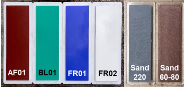
(a) Test panels coated with different fouling control coatings and sand grit.
