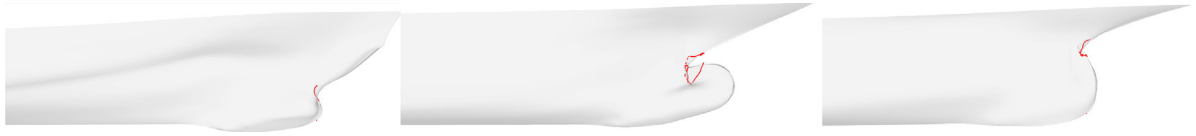
Fig. 22. Examples of invalid (self-intersecting) designs resulted from the GAN model. The red curve indicates the regions of intersection.
