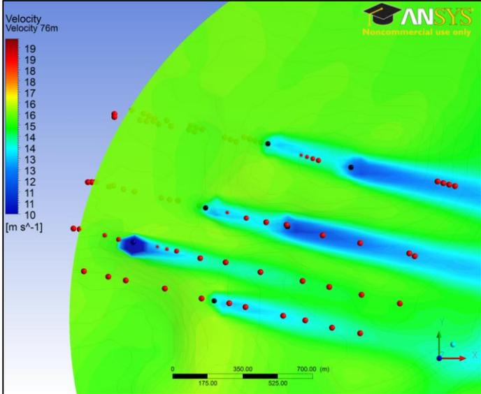
Figure 5: CFD simulation,  $k-\epsilon$  turbulence model [9]
