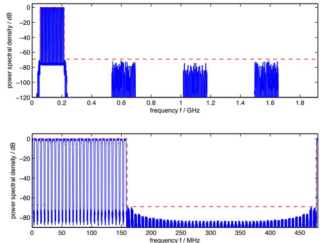
Fig. 13. Power spectral densities of stage 1 (top) and stage 2 (bottom) signals, with spectral masks indicated as dotted lines (US-1).
