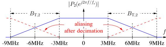
Fig. 7. Stage 2 (US-1,2) prototype filter with 6MHz passband width and decimation to 12MHz sampling rate.
