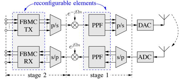
Fig. 2. Proposed reconfigurable TVWS filter bank transmitter (above) and receiver (below) with a polyphase filter (PPF) in stage 1 and a FBMC modulator in stage 2.
