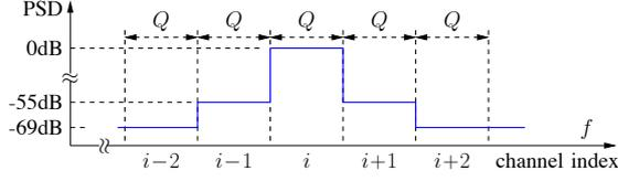
Fig. 1. Spectral mask defining permitted PSD levels in adjacent ( $i \pm 1$ ) and next-adjacent 8MHz TVWS channels ( $i \pm 2$ ) [1].  $Q = \{6,8\}$ MHz according to configuration.
