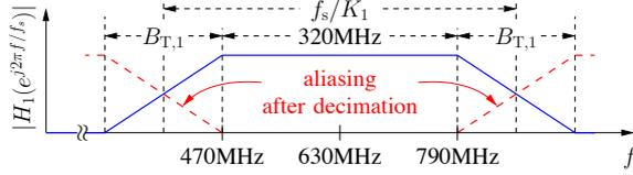
Fig. 3. Stage 1 (UK-1) filter characteristic with passband of 320MHz to capture the TVWS spectrum, and transition bandwidth  $B_{T,1}$ .
