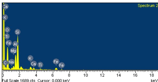
Figure 10. EDX spectra of a sample (mainly soil)
