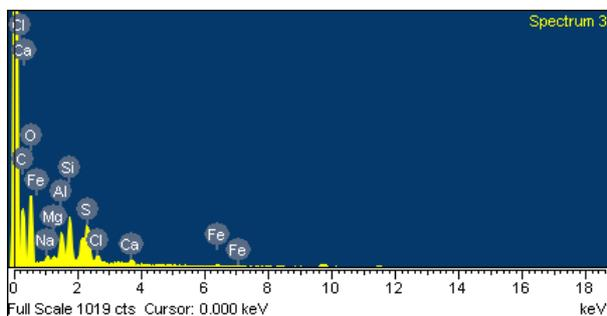
Figure 11. EDX spectra (soil and alginate particle)
