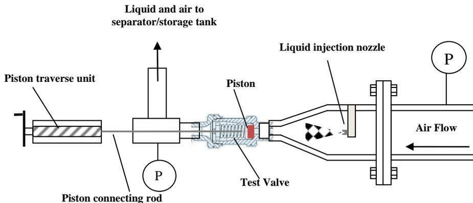
Figure 3 Schematic of valve two phase test facility
