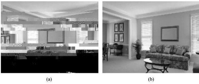
Fig. 3 Sample of a decoded images (Joint Photographic Experts Group) from the experiment for Q = 100 and SNR 10.45 dB: (a) classical and (b) quantum
