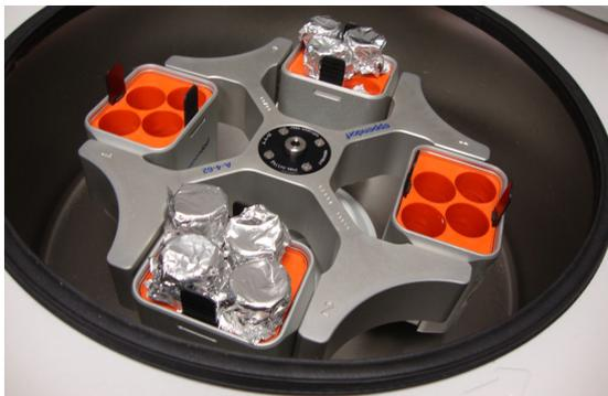
**Figure 2: Preliminary Testing of the Asteroid Analogue Target Material in the Sigma Centrifuge at the University of Glasgow**
