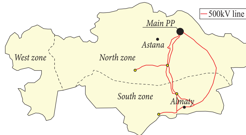
Figure 2. Simplified North-South electric power transmission network of Kazakhstan National Power System (PP—power plants, the system operator divides the NPS into three zones).
