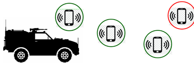
Fig. 1. Background in defence: in the presence of stationary users (in green) we would like to detect an emerging transient source (in red) which could represent a mobile phone signal triggering an improvised explosive device. (For interpretation of the references to colour in this figure legend, the reader is referred to the web version of this article.)
