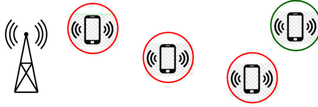
Fig. 2. Background cognitive radio: in the presence of secondary users (in red), the aim is to detect an emerging primary user (in green), such that secondary users can vacate the frequency band. (For interpretation of the references to colour in this figure legend, the reader is referred to the web version of this article.)
