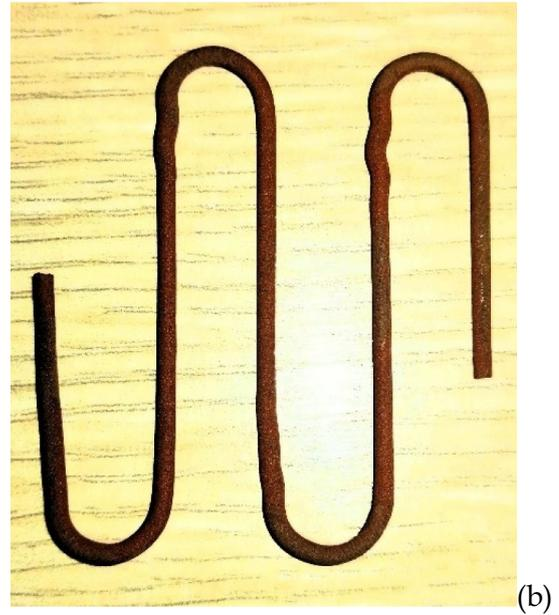
Fig. 6 Trajectory of the deposited tubes with  $R/OD=2.1$ ,  $X$  and  $Y$  axes in mm (a); example of a green copper serpentine with  $R/OD=4.2$ , deposited at extrusion velocity  $V_e=5$  mm/s, work table
