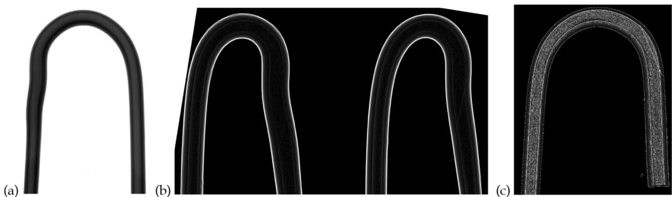
**Fig. 7** Black and white detail image of a deposited PP tubes with  $R/OD=6$  (a); details of outer profile of two tubes with  $R/OD=3$  after edge extraction with the software Image J (b); inner profile of a tube with  $R/OD=6$  after edge enhancement (c)
