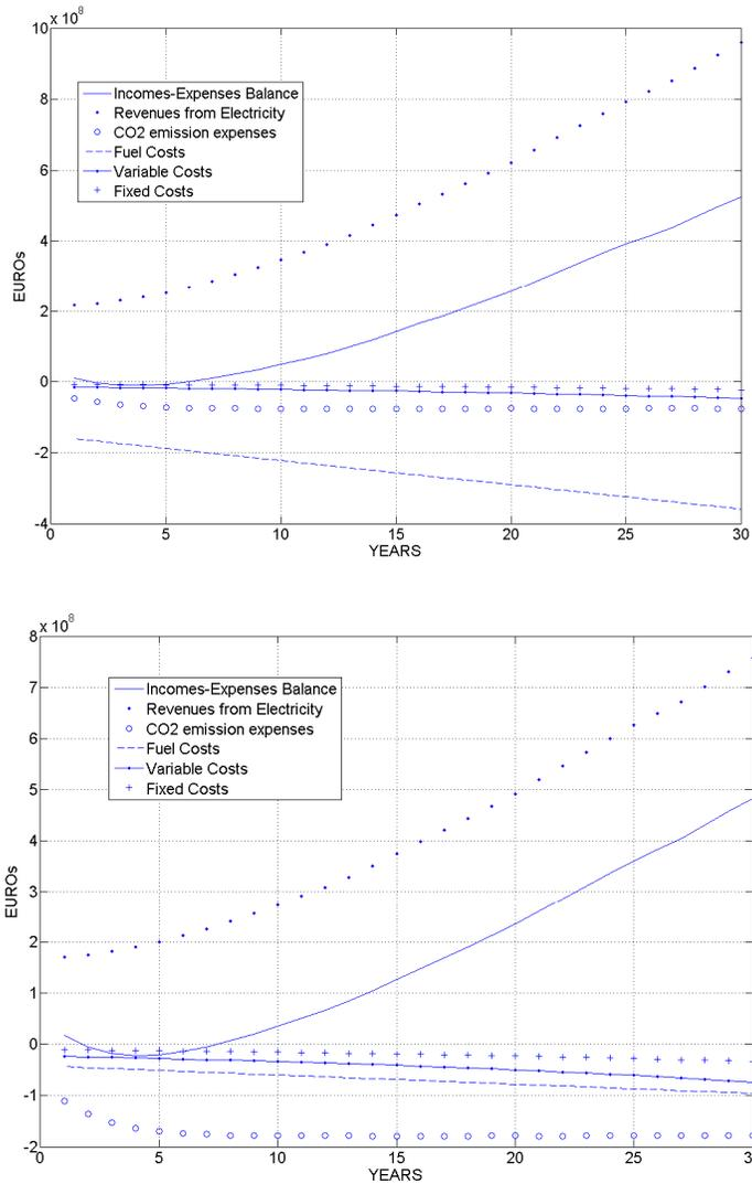
**Figure 3.** Structure of incomes and expenses for a natural-gas (up) and new lignite (down) plant
