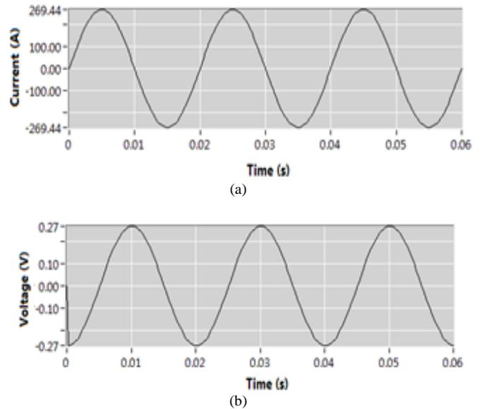
Fig. 5. Simulated Rogowski coil signals (a) primary (fault) current, (b) open circuit emf.
