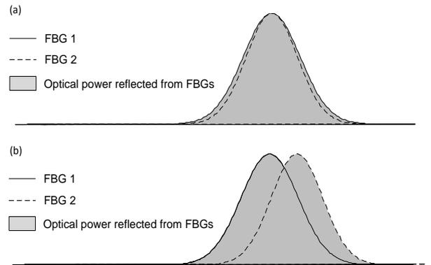
Fig. 3. Optical power distribution between two FBGs: (a) FBGs are aligned; (b) FBGs are spaced apart.
