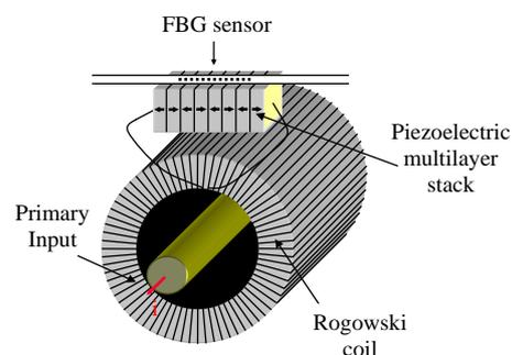
Fig. 1. Optical current sensor employing a Rogowski coil and an optical voltage sensor.
