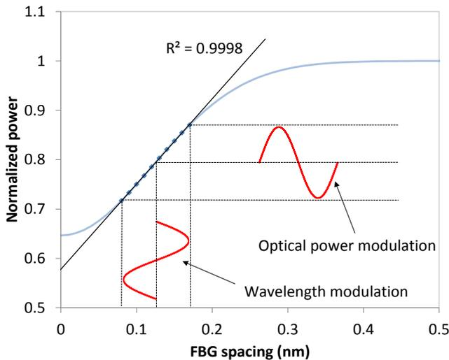
Fig. 4. Normalized optical power levels versus FBG spacing for two FBGs having equal bandwidths and reflections.
