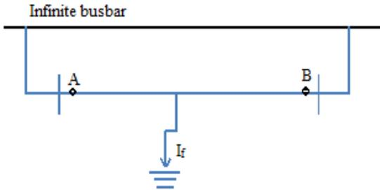
Fig. 2. Differential protection on a two ended circuit.
