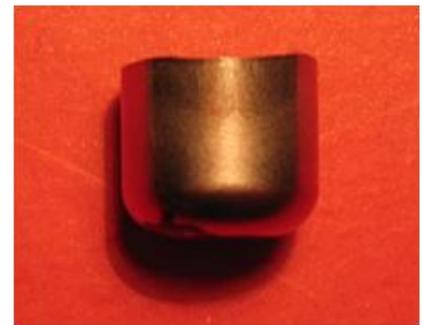
Fig.5 Shape formed in the first drawing operation.
