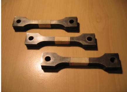
Fig.2 Packs of tensile test specimens.
