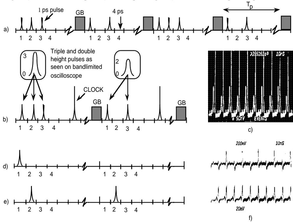
Fig. 4. Timing diagram. a) Two optically compressed packet headers "111" and "101"; b) Polarization multiplexed packets and clock; c) Oscilloscope trace of b); d) TOAD1 output after demultiplexing address bit 1; e) TOAD2 output after demultiplexing address bit 2; f) Oscilloscope trace of d) and e).
