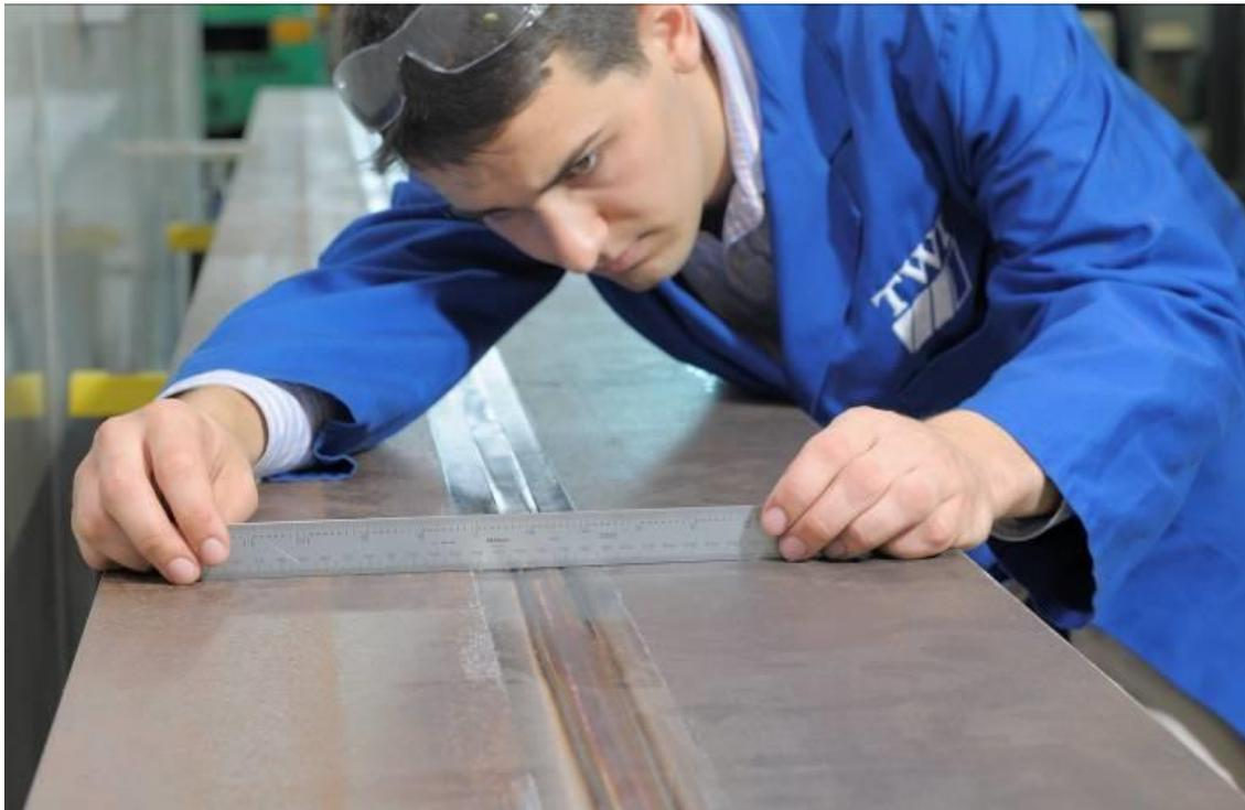
**Figure 3** Single pass friction stir weld in 6mm thick carbon steel
