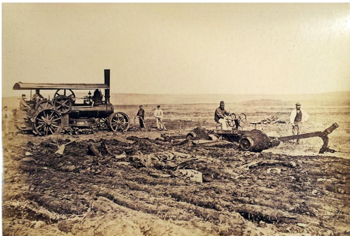
Figure 2: Steam ploughing in Sutherland (the 3 rd Duke is seated on the plough) 30
