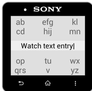
**Figure 1:** Prototype smartwatch text entry on Sony SmartWatch 2
