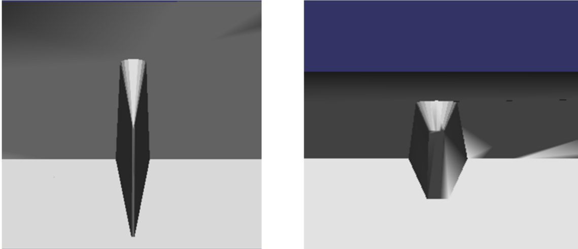
Figure 9 Simulation of FIB machining using a haptics-based program. The cross sectional dimensions are acquired from the experimental data shown in Figure 8.
