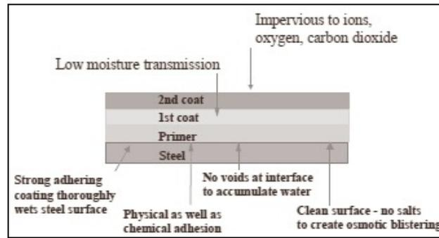
Fig. 7 An impervious coating system [4]
