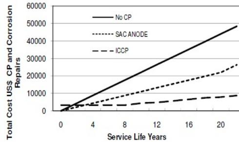
**Fig. 6** Cost comparison of cathodic protection (per 100 m<sup>2</sup> of underwater steel) [9]
