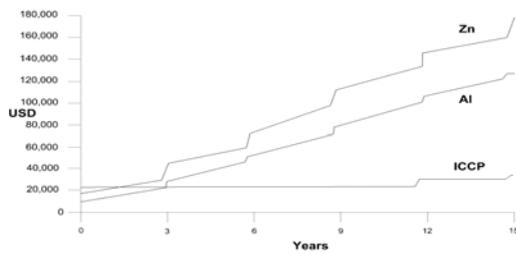
**Fig. 5** Life cycle cost for a Panamax with wetted area circa 9000 m<sup>2</sup> [7]
