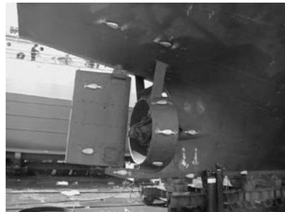
**Fig. 4** A typical installation of anodes around the stern of a ship [8]
