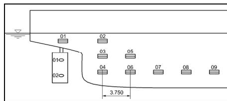
**Fig. 9** Anode distribution of the vessel around the stern
