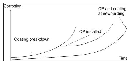
Fig. 8 Corrosion vs. time curves in different corrosion protection methods [4]
