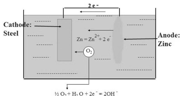
Fig. 1 A corrosion cell [4]
