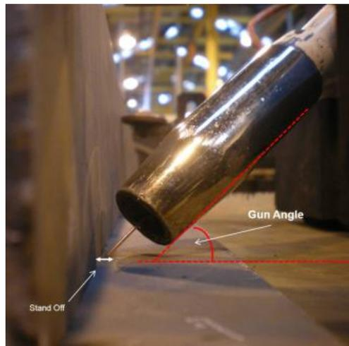
**Figure 6 : Image showing gun angle and stand-off measurement**
