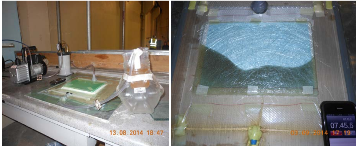
Figure 2. Vacuum Infusion Setup – Recycled Glass Fibre/Polyester Resin Laminates
