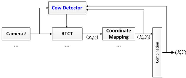
Fig. 4. Modified cow tracking with Cow Detector
