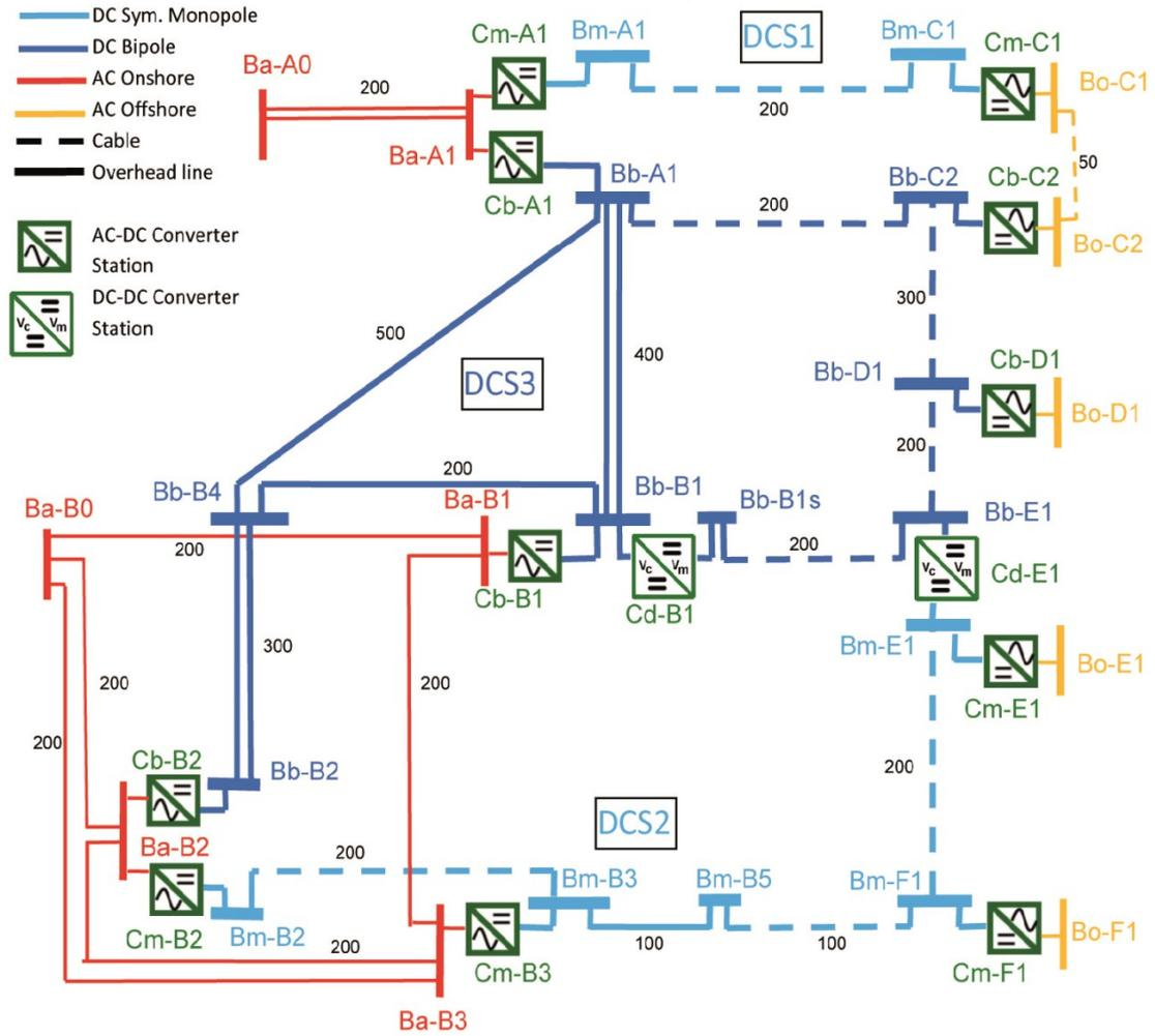
Figure 24: The CIGRE B4 DC Test Grid
