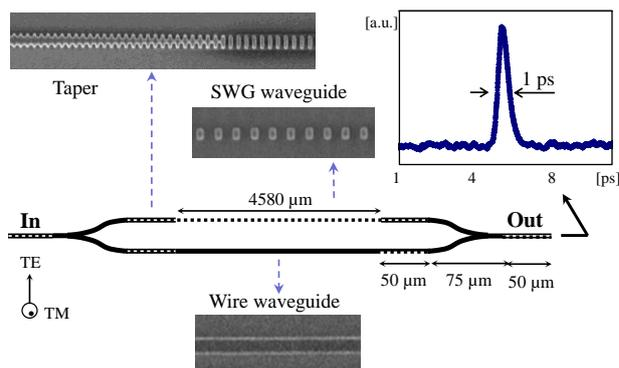
Fig. 5. A terabit all-optical self-switching device based on the Mach-Zehnder interferometer. The inset illustrates 1Tbit/s switching capabilities of this device; SWG is subwavelength waveguide grating structure
