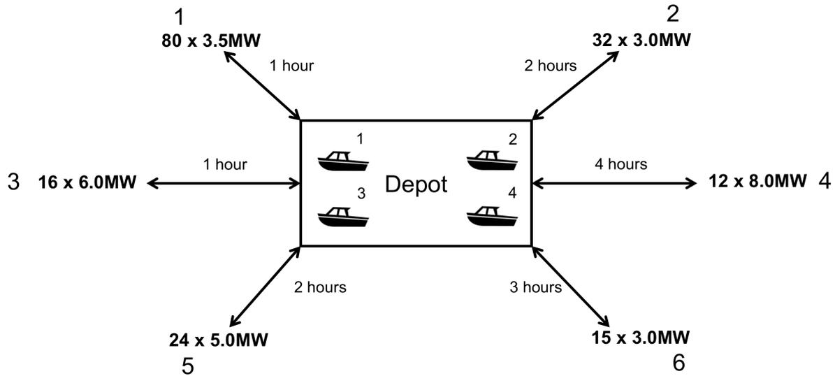
**Fig. 2.** Example central dispatch simulation, showing 6 offshore wind farms of varying installed capacity and model type, dependent on one onshore maintenance depot with 4 dispatchable maintenance teams.
